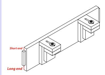
Notice placement of wood tongue. It is not center. When sliding into the groove in step 5, the short side is down.
