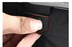
\*Press and hold the bumps on the side roof board and take out the front and rear roof. (if it is the roof board on the side of the mop, the mop shall be lowered first to pull out the buckle before taking out the roof board)
