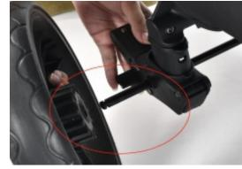
Lift the front wheel quick release button, install the front wheel and push it to the bottom.
