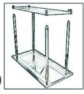
After all four pipes have been Attached, lower the adjustable Table base and let each pipe Into the base holes.
