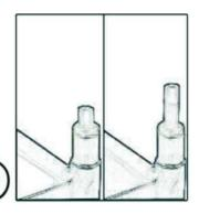
All four pipes can be adjusted for The surfaces.that are not completely level.Rotate the plasstic foot pad for differences in floor surface.
