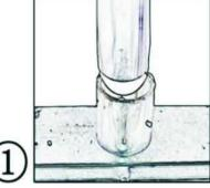
Let the tabletop upside down on a soft clotin to prevent scratches. Insert one pipe into a comer support.
