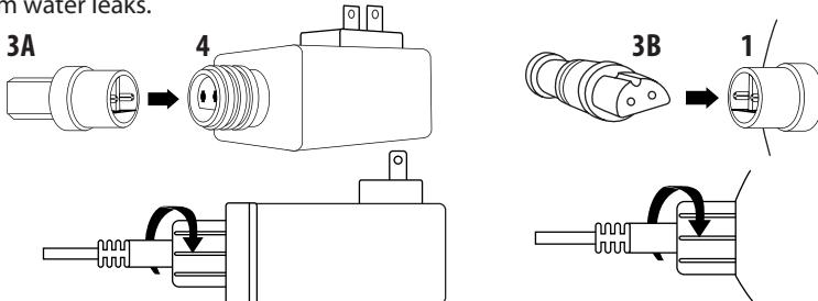
2. Plug the wall power adapter to a 110/120V power outlet that is leak safe and suitable for outdoor use.
