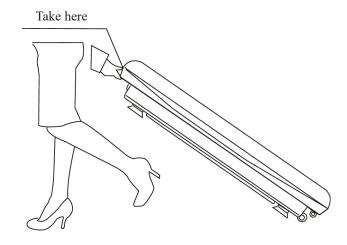
There are holding spaces under the middle cover on the both sides of the product. You can take the holding space and lift the product on 45° degree, then use the wheel to move the product to the place you want.
