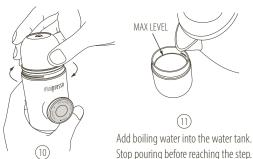
Screw tightly the outlet head
