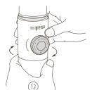
Screw tightly the main body onto the water tank until the stop.
