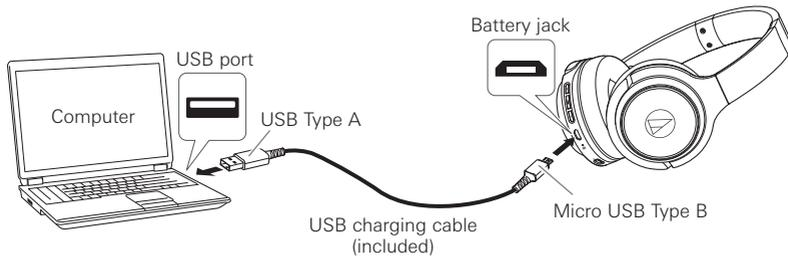
2. Connect the included USB charging cable (USB Type A side) to the computer to start charging.
