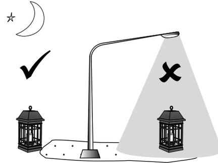
Do not position under bright light as this will prevent the light switching on at night.
