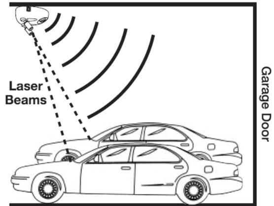
6. When you or either of your cars first enters the garage, the motion detector will turn on both lasers and the built-in light. This provides light anytime there is movement so you never have to worry about tripping in the dark or not being able to see where you are going. Drive forward until the laser for your vehicle hits your pre-determined spot indicating you are parked in the correct position. Both lasers will turn off automatically after you are parked or you have left the garage.
